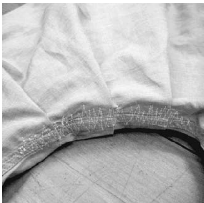
10. and make a wild zig-zagging with the straight seam to put all pleats together.
